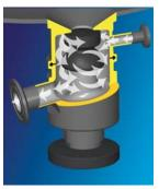
During CIP/SIP all surfaces are readily accessible by cleaning solutions, and drain completely. Optional inlet offset can enhance internal vortex flow for greater scouring action.
